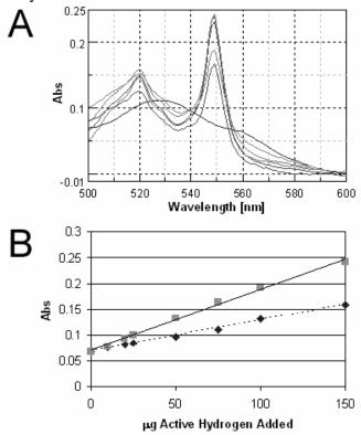
Figure 8. Cytochrome *c* analysis by spectrophotmetry. The raw spectra acquired (A) of the cytochrome *c* protein in its fully oxidized state and progression towards full reduction with spectral maxima for the reduced protein at 520 nm and 549 nm. The extrapolation data (B) indicate a linear relation ship ( $R^2$ =0.998) between the active hydrogen added and the absorbance.
