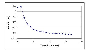
**Figure 5. ORP as a function of time with added active hydrogen.** The addition of 250 mg active hydrogen into 250 mL of distilled water resulted in a logarithmic relationship between the decrease in ORP reading and the time elapsed. In all replicates a small Gibb's free activation energy had to be overcome before the decrease in ORP.
